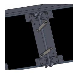
**Step 4**: Pull bracket to lock into opposing chair. Squeezing the legs together may make locking easier.
