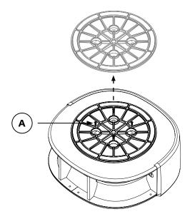
**B.** Knock the mounting plate out from the swivel base. Note: this step is made easier by propping the swivel base up on two sides so that the mounting plate is elevated above the work surface. Remove felt glides from swivel base prior to recycling.
