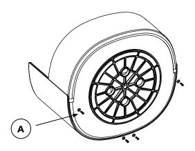
**B.** Return chair to upright position and remove the remaining H3 screws and H4 washers (x4) from the top of the plinth. Pull shell backward to release.
