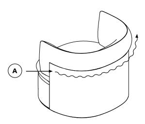
B. Untoggle the seat cushion's elastic loops from the H1 cleats, located on the left and right side of the shell interior. Release the seat cushion from the plinth. Remove H2 screws to seperate the H1 cleats from shell.
