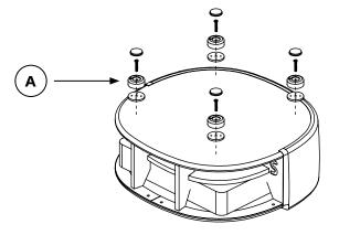
B. If your chair is equipped with casters, remove the H9 screws (x4) located inside each caster housing (x4). Once the casters are removed, release the caster housing (x4) by prying off from the plinth.
